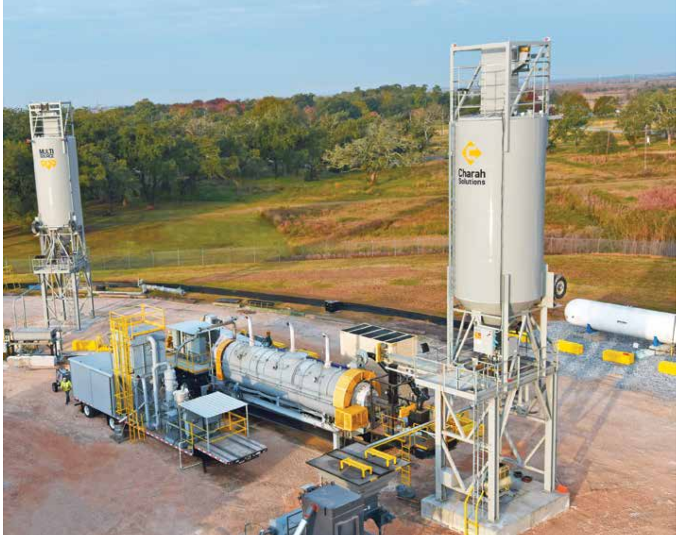
Charah Solutions' proprietary MP618® Multi-Process ash beneficiation technology converts fly ash that is otherwise unusable into a consistent high-quality fly ash that meets industry specifications.
